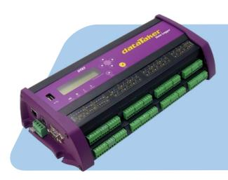
the oil wells, and USB memory stick support is included for easy data and program transfers. Advanced alarm capabilities ensure that any increase or decrease in temperatures is detected and reported as they happen, making for a safer and more productive work environment as well as better oil well monitoring.
