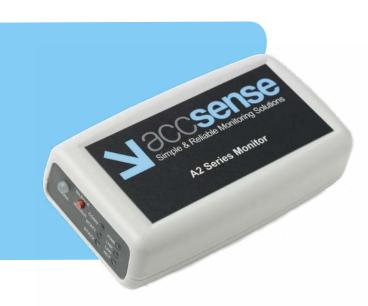
Accsense is also ideal for monitoring ultra-low supplies stored in medical freezers down to -200°C (-328°F) using the optional Type T thermocouple probe.
