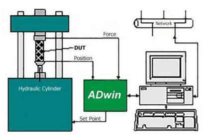
ADwin is a highly flexible and cost-effective DAQ solution for control of all kinds of vibration test stands. At CAS DataLoggers our customers especially appreciate its operational reliability even when used together with a Windows PC.
