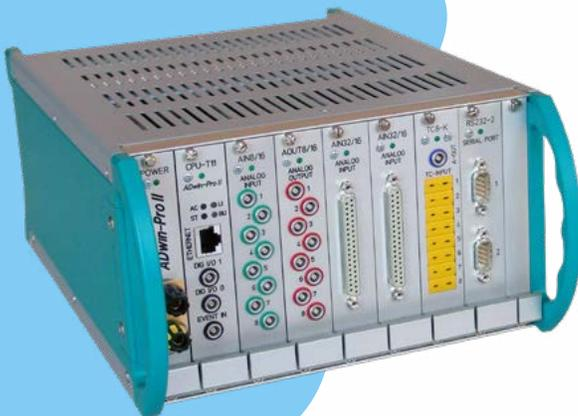
The lead test engineer contacted the North American ADwin distributor, CAS DataLoggers, who supplied an [ADwin-Pro-II Data Acquisition and Control System](#). This system is installed within a control cabinet in the automotive test lab, fulfilling the need for connection to the airbag ECU, for current stimulation to accelerometer sensors, and for SPI interface simulation.
