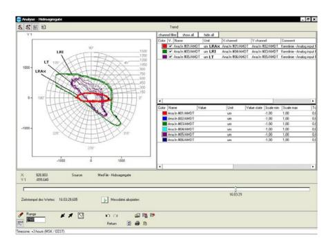
In conclusion we can say that the machine diagnosis of those machines which have journal bearings in their assembly are done more precisely if the vibration measurements are done with proximity transducers and are acquired using the on-line mode, simultaneously on all the machine's bearings. For this purpose the Expert Vibro was ideal here and the customer was very satisfied post-installation.
