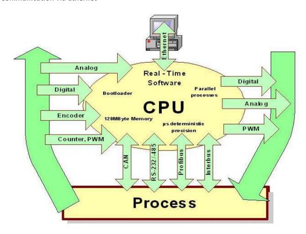
The Simatic Fetch/Write communication over the Ethernet network is a one-to-one connection between an ADwin system and a Siemens Simatic PLC. The connection allows read and write accesses to system memory areas of the Simatic. There are ways to access data blocks, flags, inputs, outputs, counters and timers.
