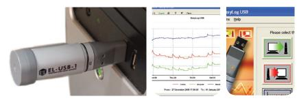
On inserting a battery the Red then Green LED will flash in turn for approximately 2 min, while the logger stabilises. Do not connect to the USB port of a computer untill this has finished.
