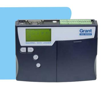
either as a stand-alone recorder or as a PC-linked data acquisition system. The SQ2020 data logger offers 8 to 16 universal analog inputs and 8 digital inputs as well as up to 16 derived/calculated channels and 4 pulse rate/counter inputs.
