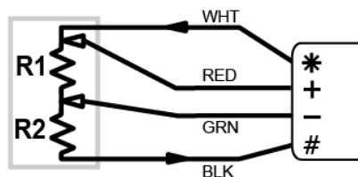
Figure 152: Wiring for 4-wire Carlson Sensor
