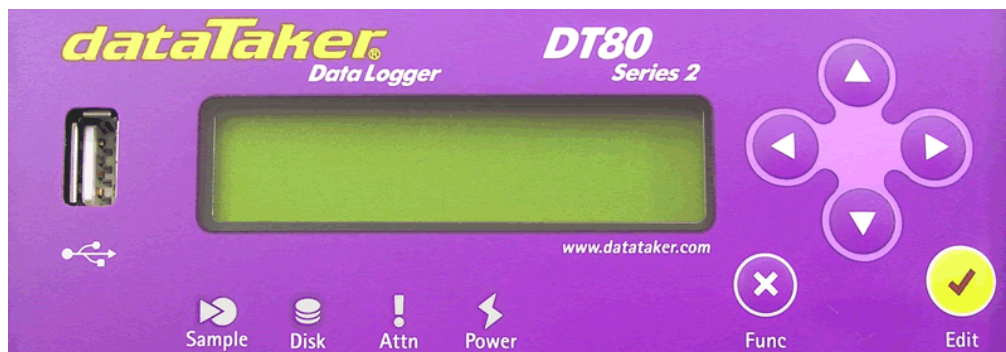
Figure 21: DT80 Front Panel
