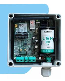
The sensor provides two Form C solid-state switches (NO, NC, COM)-one for motion alarm and one for tamper alarm. The sensor outputs are wired to the DI1 and DI2 BSC-50E digital inputs. The Normally Open terminals are used for this purpose in order to save power, as the BSC-50E inputs feature an internal pull-up resistor. An ON-OFF switch, wired to BSC-50E DI3, is used to enable or disable the GSM alarming (Arm/Disarm switch).
