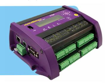
At this stage of the prepreg manufacturing process, to ensure an evenly-heated product, technicians place multiple thermocouple temperature sensors into the fiberglass mold at many different points. Then the steam-heated molds close over the material and the thermocouples (typically Type K) log the resin temperature. The temperature sensors send their data to the dataTaker data logger for storage in
