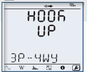
Hook up, voltage and current ratios and aggregation period can be configured from the front panel of the PEL 103.
