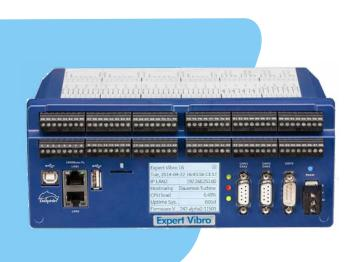
rates; up to 50 kHz per channel. Meanwhile, the system's 24-Bit A/D converters ensure high precision. Users can switch between voltage measurement, IEPE or shaft vibration sensors.
