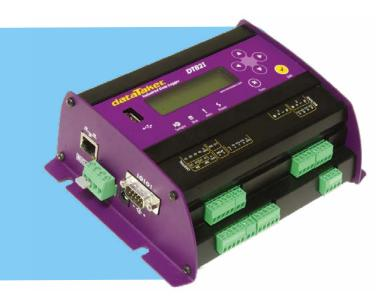
Users can overwrite or finish logging once allocated memory is filled, archive data on alarm event, copy to USB memory and transfer via FTP which provides data via an Ethernet network or mobile phone network. With dataTaker, users don't need separate polling or specific host software.
