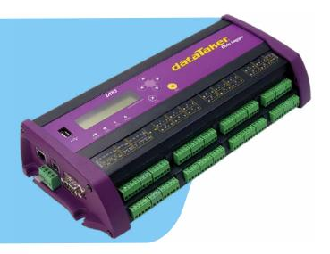
Additionally, whenever power interruptions occurred, the dataTakers generated a record of the temperatures, allowing engineers to determine exactly how much of the <u>heat</u> <u>treating cycle</u> had been completed. This reduced scrap product, lowered the building's wasted energy and helped increase product quality. The dataTakers also archived data on alarm event, sending data an Ethernet network without needing polling or specific host software.
