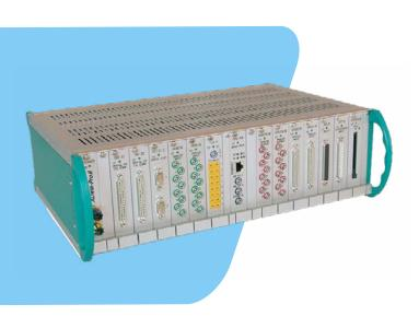
after each sample was taken. The system also handled complex triggering conditions, high analog sampling rates, and freely programmable mathematical operations and functions including RMS values, min/max, mean, derivative, digital filters, and frequency domain signal analysis.
