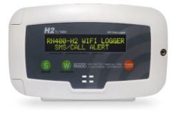
RN400-H2PS is designed to measure internal Temp/RH, and external NTC Temperature sensor signal and transfer them to the destination via WiFi connection. The destination would be an information system such as public cloud, local server, and even PC. It operates with battery power and has a protective gasket for various industrial sites. Premium RN400 H2 series have IP65 for protection, OLED screen for cold outdoor, F-RAM memory for instant backup and micro-SD card for CSV backup.
