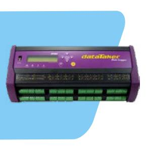
The DT85's 16 analog input channels allow 16, 4 wire sensor inputs for sensors like strain gauges or up to 32 isolated or 48 commonly referenced, 2-wire analog inputs. These inputs can be used in many combinations and support a wide variety of sensor types. The logger can store up to 10 million data points in internal memory allowing weeks or months worth of data to be stored locally. Users could also easily copy it to a USB stick or automatically send it to a server via FTP.
