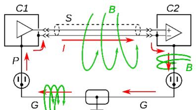
**Figure 1**. Changing magnetic field causes current in the shield and low side of signal conductor, inducing a voltage offset error in measurements
