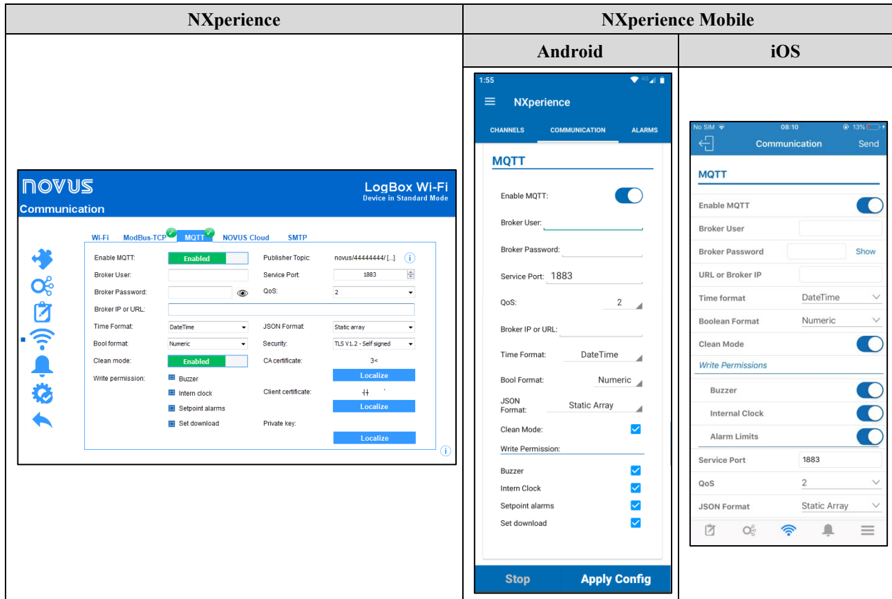
Figure 20 – Configuration Screen: MQTT
