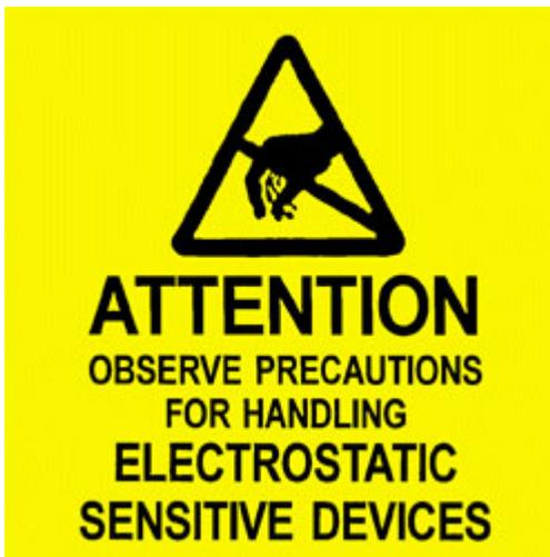
Electronic components are sensitive to ESD (**E**lectro-**S**tatic **D**ischarge). Therefore, discharge any electrostatic energy before opening the device, for example to install an I/O module or to replace the integrated memory card. We recommend wearing an anti-static wrist band (static discharge wrist band) and to carry out the work on a conductive surface.
