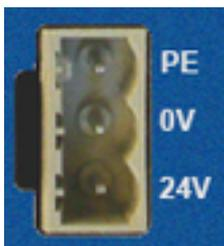
Input voltage: 12 VDC – 24 VDC ±10%
