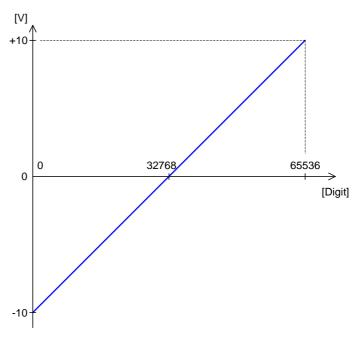
Fig. 8 – Zero offset in the standard setting of bipolar 10 Volts
