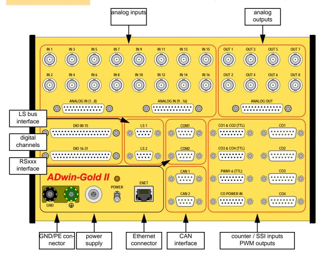
Fig. 4 - Schematic of ADwin-Gold II
