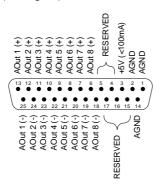
Fig. 12 - Pin assignment ANALOG OUT of DA add-on
