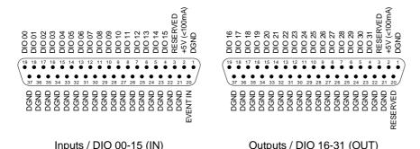
Fig. 10 - Pin assignment of digital channels
