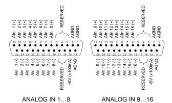
Fig. 5 – Pin assignment of analog inputs (DSub)
