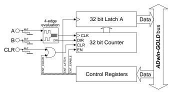
Fig. 18 – Block diagram CNT add-on in mode "four edge evaluation"
