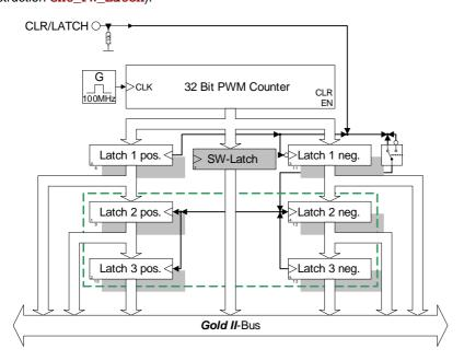
For any evaluation the PWM register of levels 2 and 3 are used. First, the register values are copied to the shadow registers with <a href="mailto:Cnt\_Sync\_Latch">Cnt\_Sync\_Latch</a> and then evaluated.
