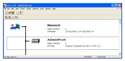
Configure number and length of input and output data of input and output data in the fieldbus node memory one by one.
