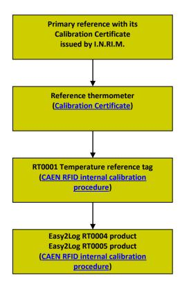
Fig. 5.1: Temperature measurement traceability chain
