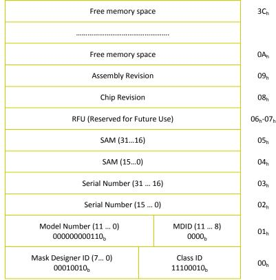
Fig. 3.1: TID memory bank structure
