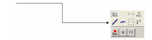
This button enables the joining of measurement points either as a smooth curve or a stepped curve. Smooth joining is the default setting. Stepped joining is necessary when the individual points require measuring out.
