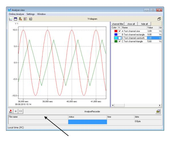
The recorder bar contains information on recordings and enables the manual start / stopping of a recording.
