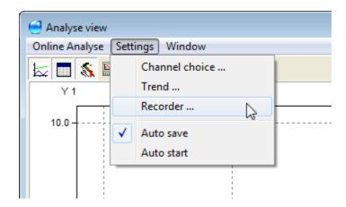
Recorder file names can be assigned using the recorder settings. The name can be a specific name.
