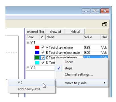
A dialogue is displayed that lists the current Y-axes to which channels can be assigned.
