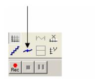
This button enables measuring points along the measurement curve to be marked with a small cross. The measurement points can be portrayed as joined or non-joined.
