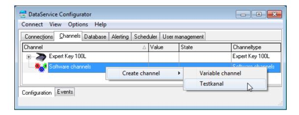
This opens a dialogue in which you can create and configure a test channel.
