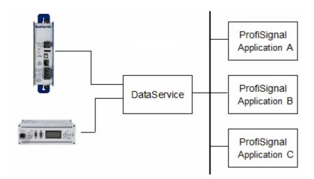
Expert devices are equipped with an USB interface and a LAN interface. Message devices are equipped with a LAN interface.
