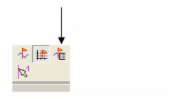
Left clicking the symbol displays a dialogue that enables markers to be deleted. With multiple markers, select the marker to be deleted.
