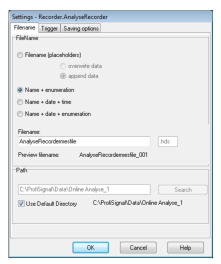
The *Filename* tab enables individual names to be automatically assigned to files. This is especially important for experiment series.
